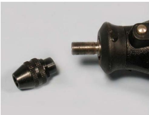
Many of us have a Dremel motor tool to use at home or when out to a class or workshop. The one thing that makes this tool much more productive is the addition of one inexpensive option, an adjustable chuck.
