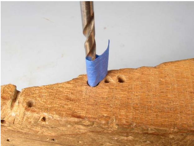
Sometimes you need to drill a number of holes all to the same depth. One quick and easy way to do this is to wind some tape around the drill bit so that the tape just touches the part surface when the hole is deep enough.
