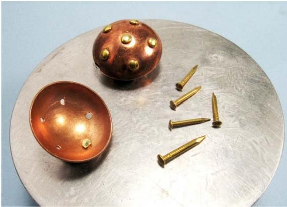
For a nice looking rivet head, use brass escutcheon pins. You'll have perfectly rounded heads that are all the same size and shape. The pins are a little hard to find, so try the best hardware stores first. Be sure to get solid brass pins, not brass plated steel. If unsure, test them with a magnet.
