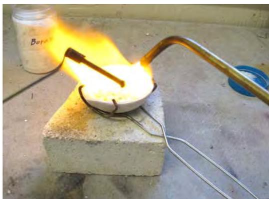
When the dish is hot, sprinkle in a half teaspoon of borax, let it melt, and spread it with a carbon rod over all of the interior surface of the dish. Add more borax if needed.
