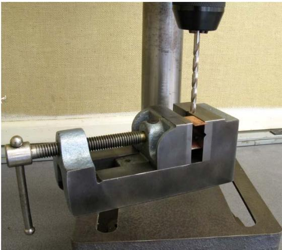
A drill press vise is a versatile tool to hold a workpiece securely and in precise alignment. It reduces the of risks of working with high power motors, use of larger drill bits, and higher heat generated in the operation. The vise can be clamped to the drill press table if needed and is quite handy for use at the bench to hold things for sawing or riveting.
